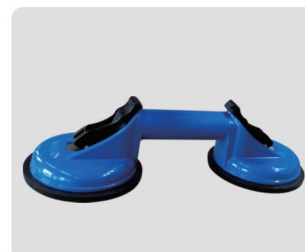
Suction Cup dia 140mm thickness 7mm 130kgs
