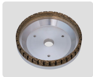
External segment beveling diamond wheel Seven star stone F3 \phi 150 \times 6 \times 12 F4 \phi 150 \times 6 \times 12 F4 \phi 150 \times 8 \times 10 Aperture:22 Granularity:100#
