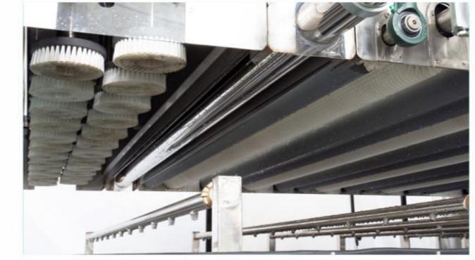
Air knife set after the disc brush zone to reduce the polishing power entering next washing zone.
