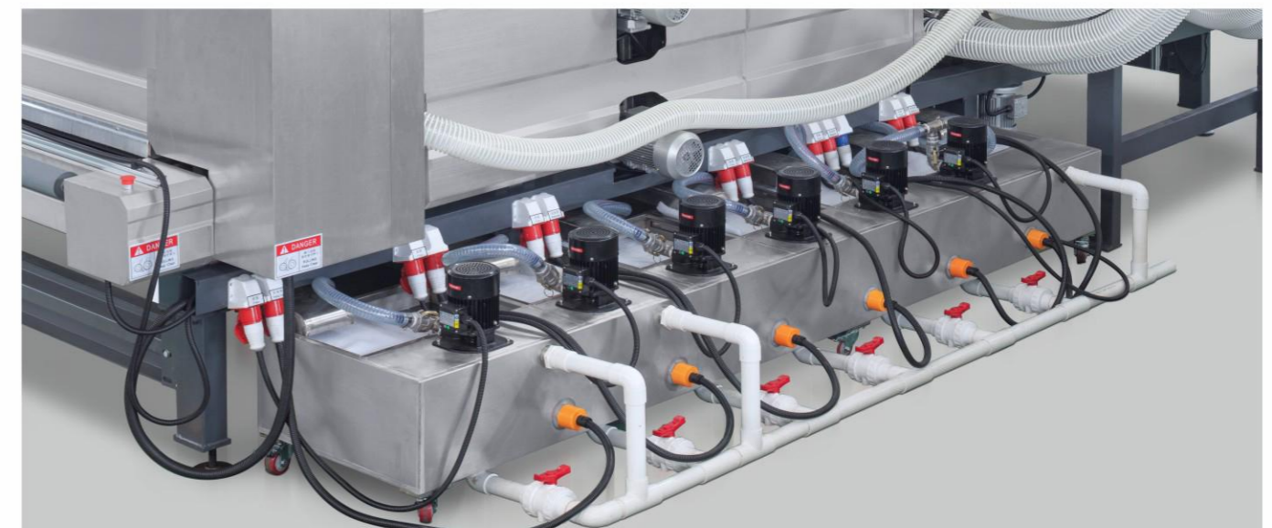
The tanks placed at the side of the machine so you can easily check if the water is clean or not. Separate water tanks with water pumps.
